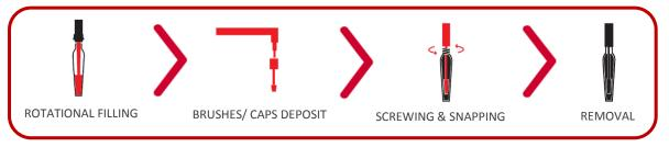
The RMAQ-60 is a **versatile** filling and sealing machine designed for the packaging of make-up and cosmetic products.
