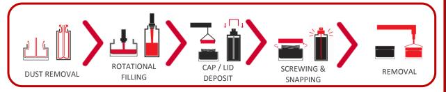
The RB-60 is a versatile machine designed for filling and capping all types of jars and bottles.
